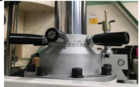
Precision Bottom Dead Centre Adjustment (in 0.025mm)
